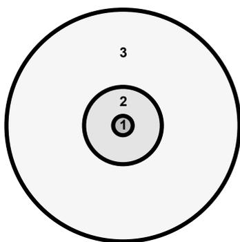
**Figure 1: The basic BioSoil plot.** Coarse woody debris, snags, stumps, ground vegetation and canopy characteristics are measured in the BioSoil subplots 1 and 2 (a total sampling area of 400 m<sup>2</sup>). Tree species and DBH (diameter at breast height 130 cm) are recorded across the entire BioSoil plot.
