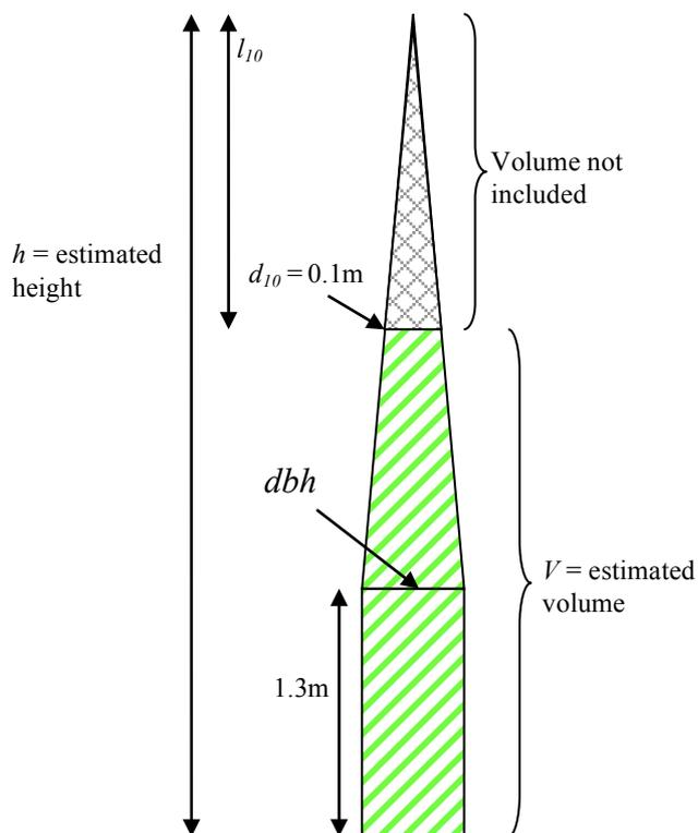
**Figure 35: Schematic representation of volume estimation of dead tree**
