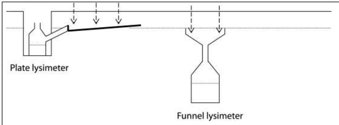
Figure 2: Examples of different types of zero-tension lysimeters.
