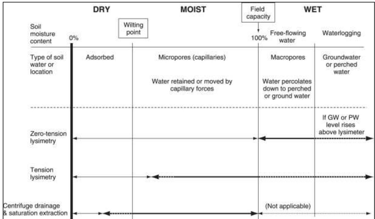
Figure A1-1: The soil water fractions sampled by zero-tension lysimetry, tension lysimetry and centrifuge drainage (thick lines). The thin lines indicate the fractions that cannot be sampled. The actual fractions sampled by tension lysimetry can vary depending on the size of the vacuum applied and the moisture content of the soil during sampling (dotted lines).
