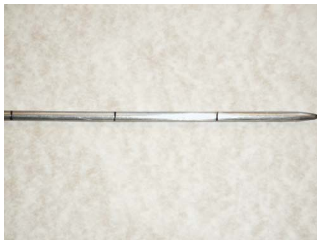
Figure 2: Tip of the penetration rod
