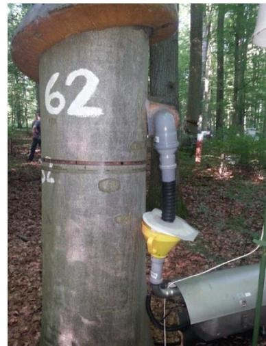
Figure 6-3. Stemflow collectors are permanently installed on the stems to collect any run-off from the branches and stem (here on *Fagus sylvatica* L.). Stemflow is, compared to throughfall, enriched in ions washed off the bark.
