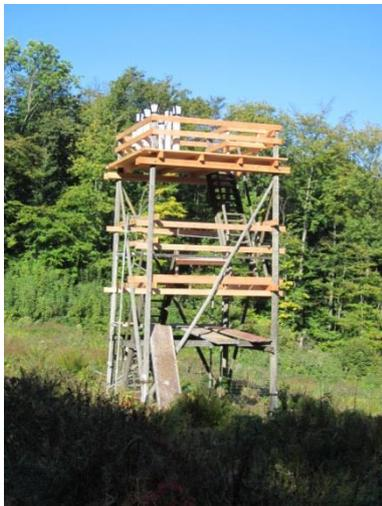
Figure 6-1. Adjacent to the forest stand open field precipitation is measured which is not influenced by the exchange processes within the tree canopies.
