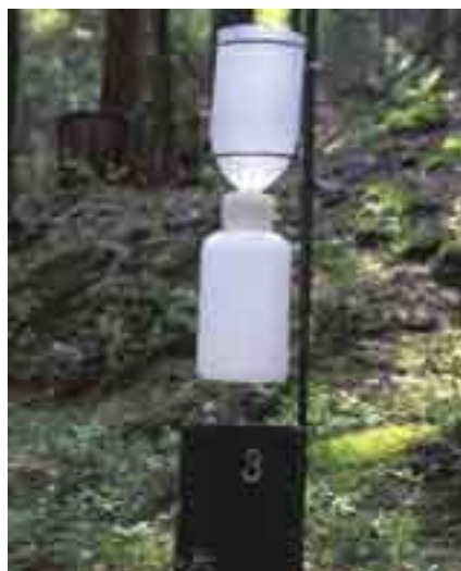
Measurement equipment for the collection of wet deposition inputs in forest stands
