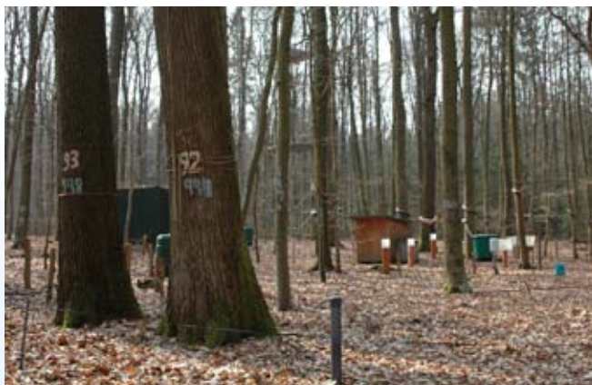
Level II plot in Germany with permanent circumference measurement tapes (foreground), throughfall and stemflow deposition samplers.
