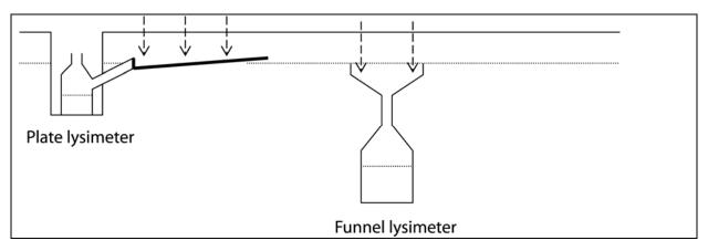
Figure 2: Examples of different types of zero-tension lysimeters
