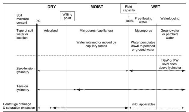
**Figure A1-1: The soil water fractions sampled by zero-tension lysimetry, tension lysimetry and centrifuge drainage** (thick lines). The thin lines indicate the fractions that cannot be sampled. The actual fractions sampled by tension lysimetry can vary depending on the size of the vacuum applied and the moisture content of the soil during sampling (dotted lines).
