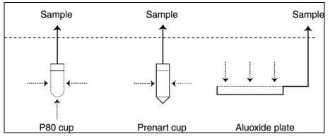
Figure 1: Examples of different types of tension lysimeters
