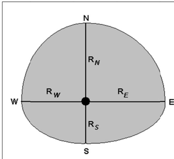
**Figure A1-4:** Measurements of crown diameter (4 radii)
