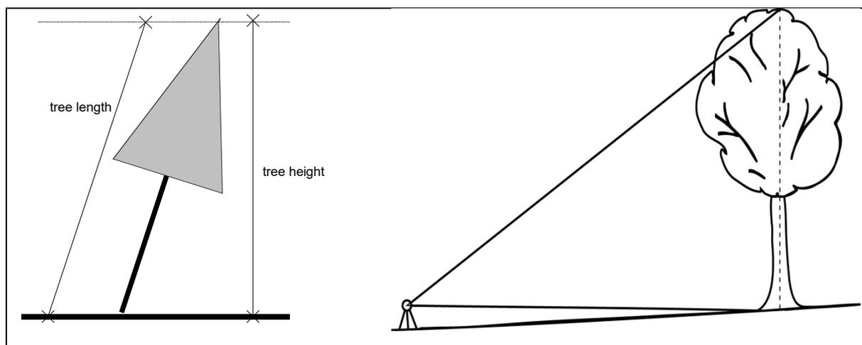
**Figure A1-3: To be observed when measuring tree height on broadleaved and leaning trees**
