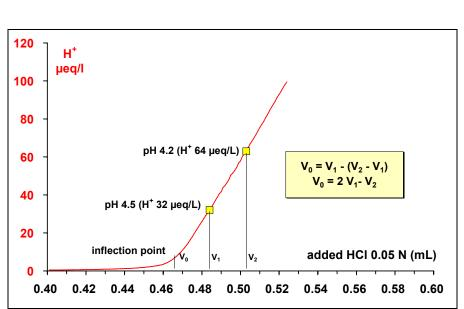
**Figure A4.2:** Plot of the concentration of hydrogen ions during the final part of an acidimetric titration, showing the extrapolation to the equivalence point, i.e. the intercept on the x-axis of the line straight line passing through the two end points.
