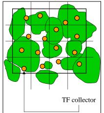
Figure 3: Combination of systematic and random sampling on the same plot or random selection of sites within previously selected equally-sized parts of the plots.
