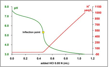
Figure A4.1: Plot of pH and hydrogen ion concentration during an acidimetric titration.
