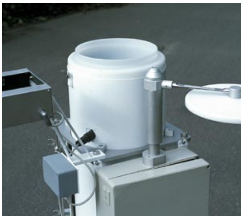
Wet only deposition sampler. In order to distinguish wet from dry deposition, these samplers open only when rain, snow or extreme fog are occurring.
