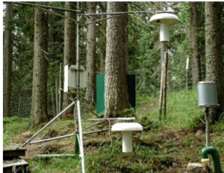
CONECOFOR Plot with meteorological station for continuous microclimate measurements.
