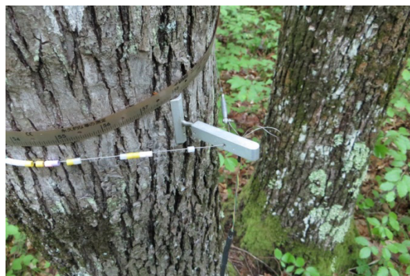
Figure 6-1: Point dendrometer – picture taken at the Romanian Level II plot in 2016; on the top of the point dendrometer a manual girth band is located (T. Levanič)
