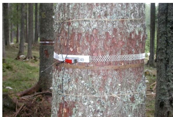
Figure 6-2: Band dendrometer with manual girth band installed below the electronic dendrometer – picture taken at Slovenian Level II plot (T. Levanič)
