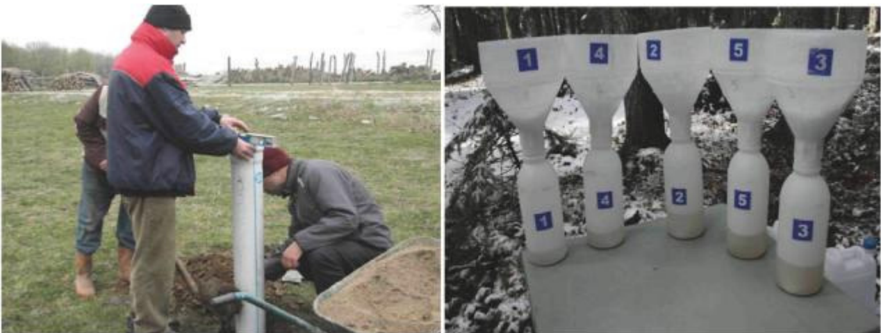
Figure 9. Installation of total deposition samplers at Level II site (left), and rain water collected in the samplers (right) (Photo: M. Zengin).
