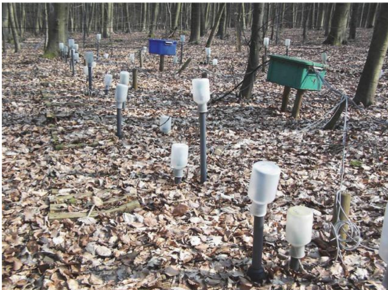
Figure 14. Sampling soil solution in a Level II observation site in Hamburg.
