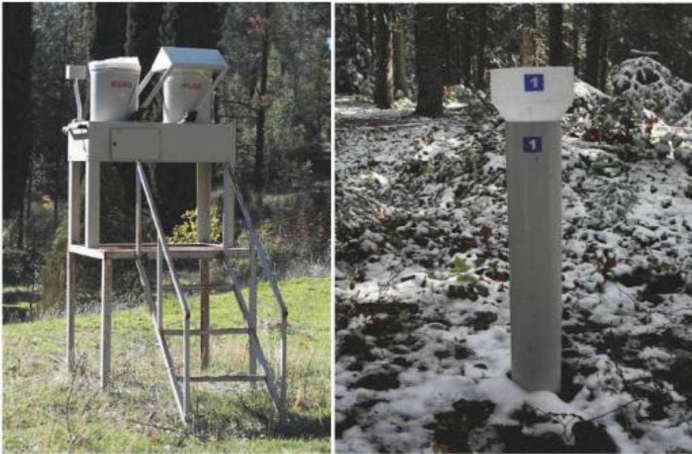
Figure 8. Dry and wet deposition samplers in the Level II observation site No. 10 (left) (Photo: D. Tolunay), and total deposition sampler in Level II observation site No. 6 (right) (Photo: M. Zengin).
