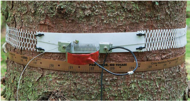
Girth bands automatically measuring changes in tree stem diameter record tree circumference growth at one-hour intervals. The time that growth begins and ceases can be determined on the basis of the recorded data. Radial increment is also monitored using manually read girth bands.
