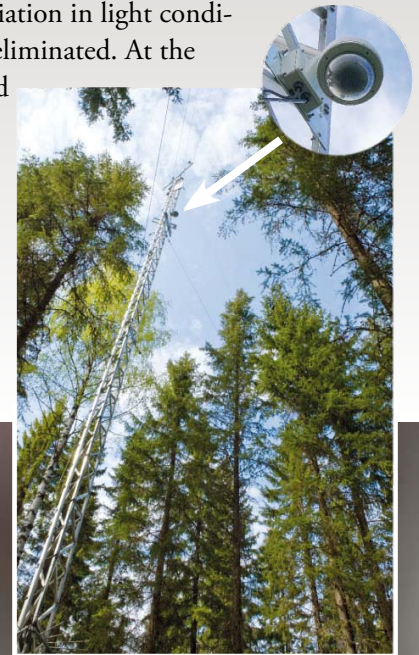
Digital camera attached to a meteorological observing station (weather tower).
