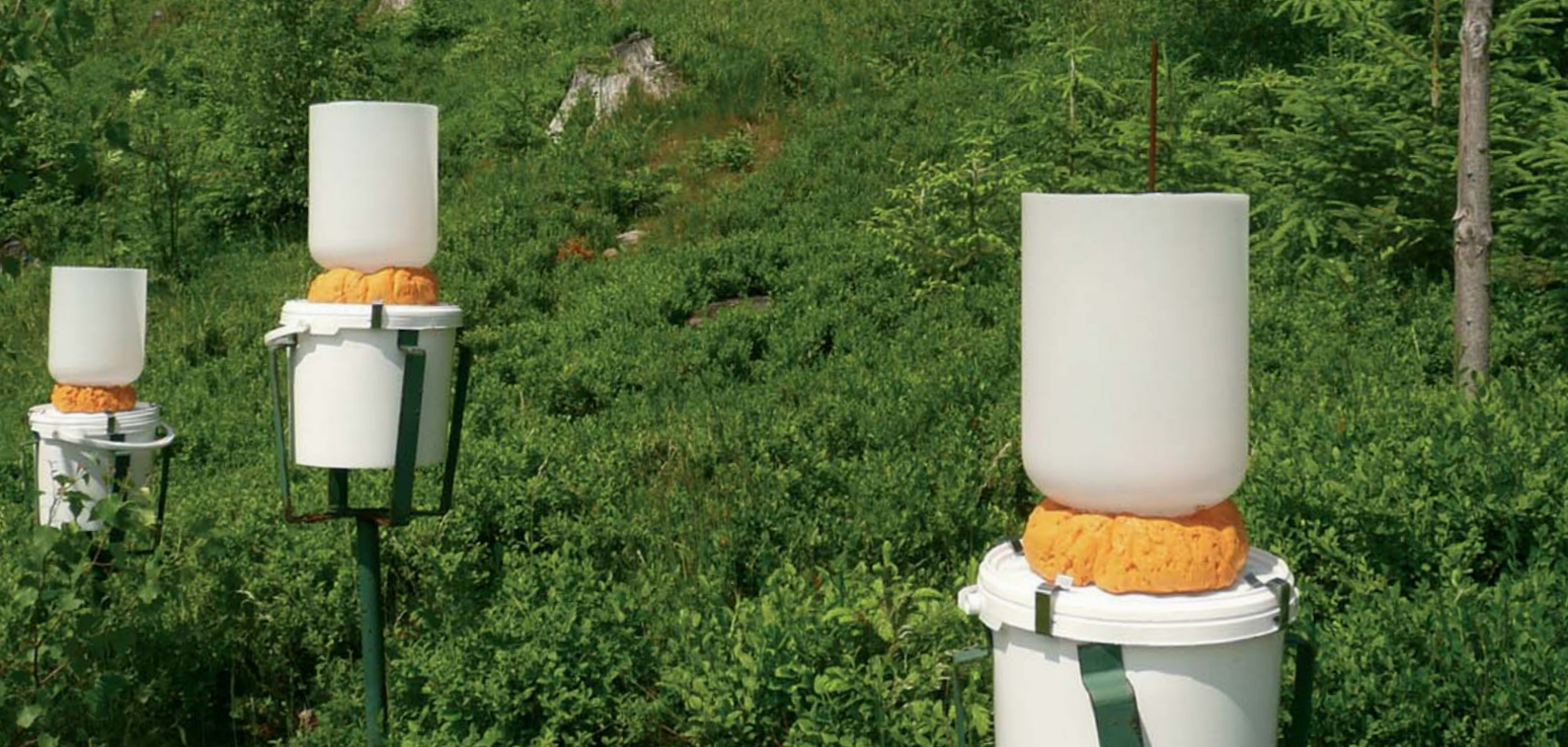
To minimise errors due to contamination, several deposition samplers are run in parallel at the open field site in Gronik, Slovakia.
