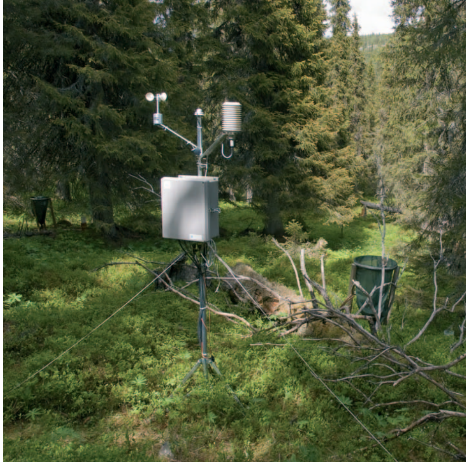
Meteorological measurement station and litterfall sampler in a Nordic spruce forest.
