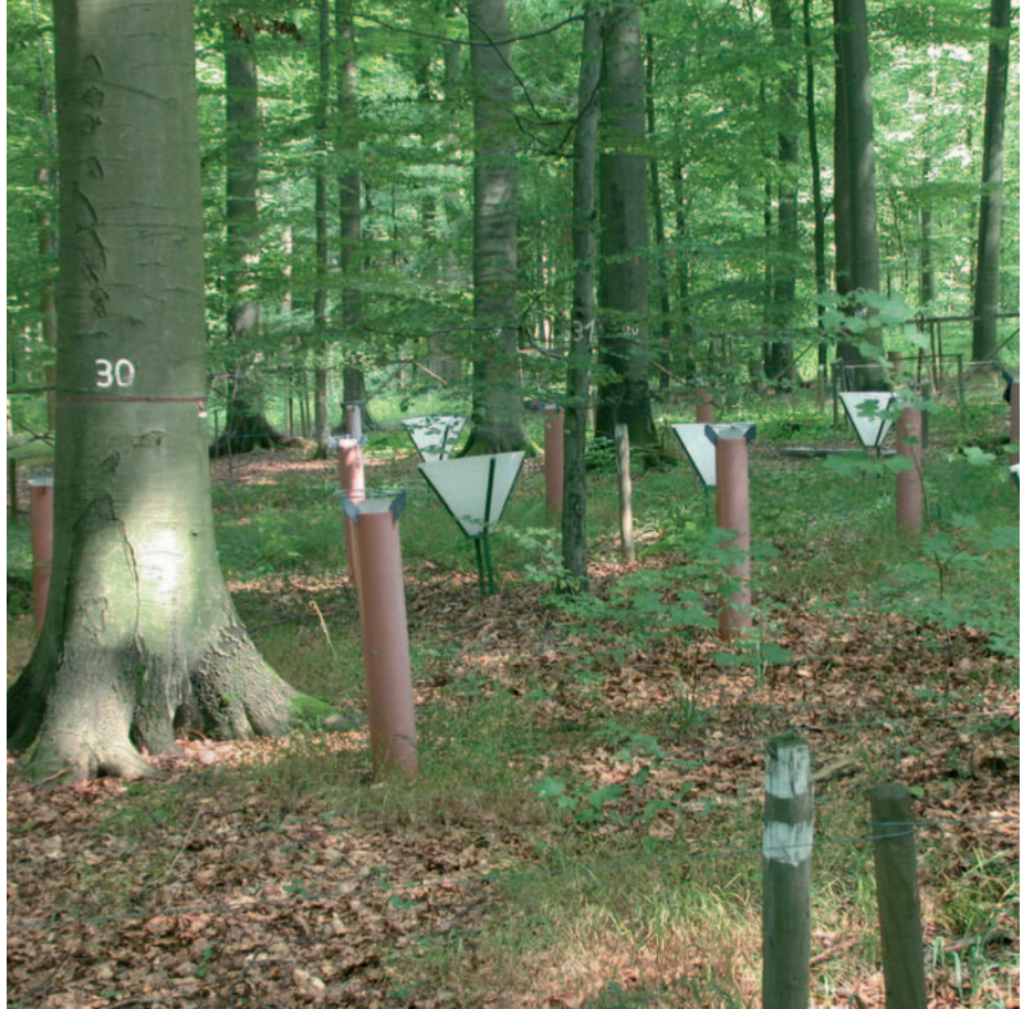
Intensive Monitoring plot in a central European beech forest with litterfall (white) and deposition (orange) samplers.
