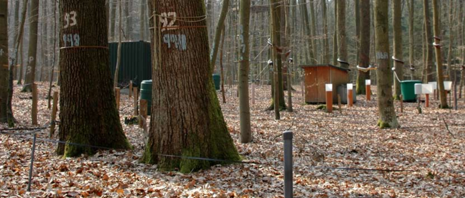
Intensive monitoring plot in Germany with permanent circumference measurement tapes (two oak trees in the foreground), throughfall samplers (three white round samplers in the middle) and stemflow collectors (green barrel).
