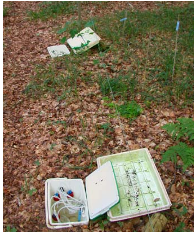
Lysimeters extract water, which is called soil solution, for analysis in the laboratory. Soil solution reacts to deposition and plays an important role in the forest ecosystem. It is, for example, essential for water and nutrient uptake by plants.
