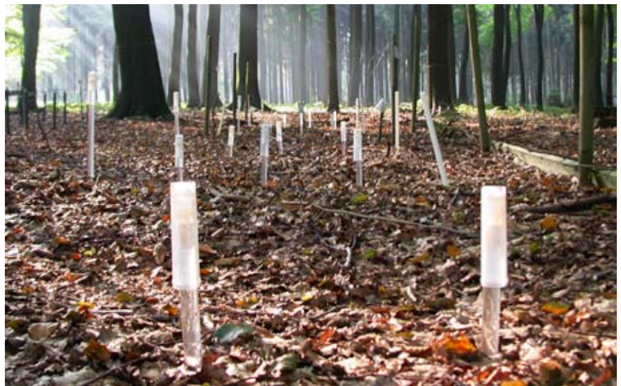
An array of soil tensiometers designed to assess the variability in soil water tension at a Level II plot in Germany.
