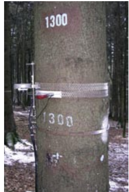
Continuous girth band measurements can measure growth changes within single years.
