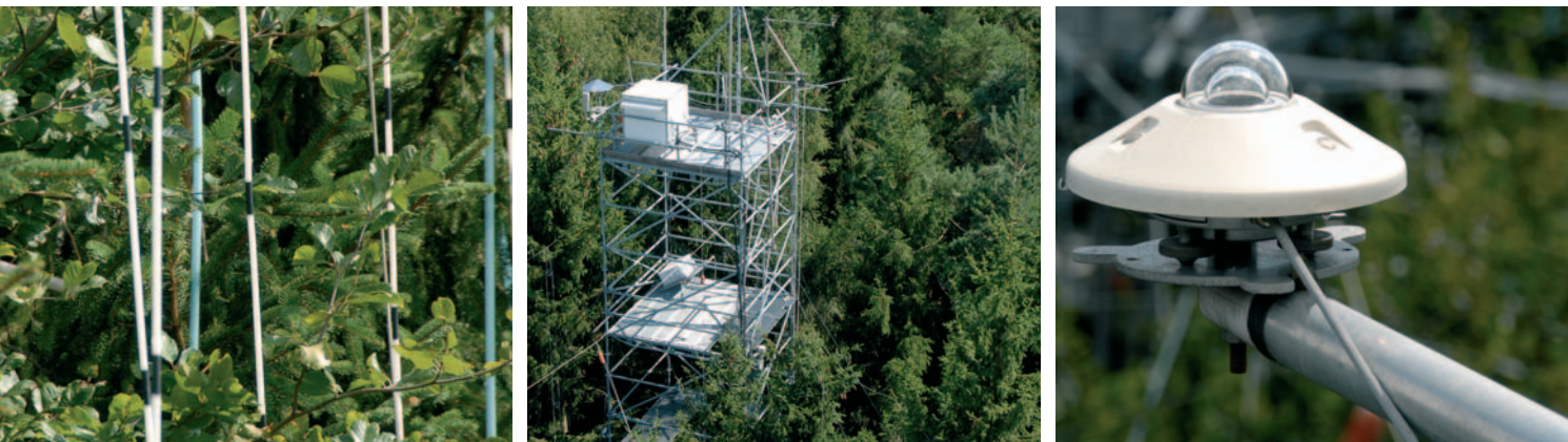
Ozone fumigation system (left), eddy-flux measurement system (middle), and radiation sensor (right) at the free-air ozone fumigation facility at Kranzberg Forest, Germany. For accurate ozone risk assessment modeling more information on real-time ozone concentrations and gas exchange is needed. Such data can be provided by free air fumigation, sap-flow and eddy-flux measurements that are combined with meteorological and soil monitoring.
