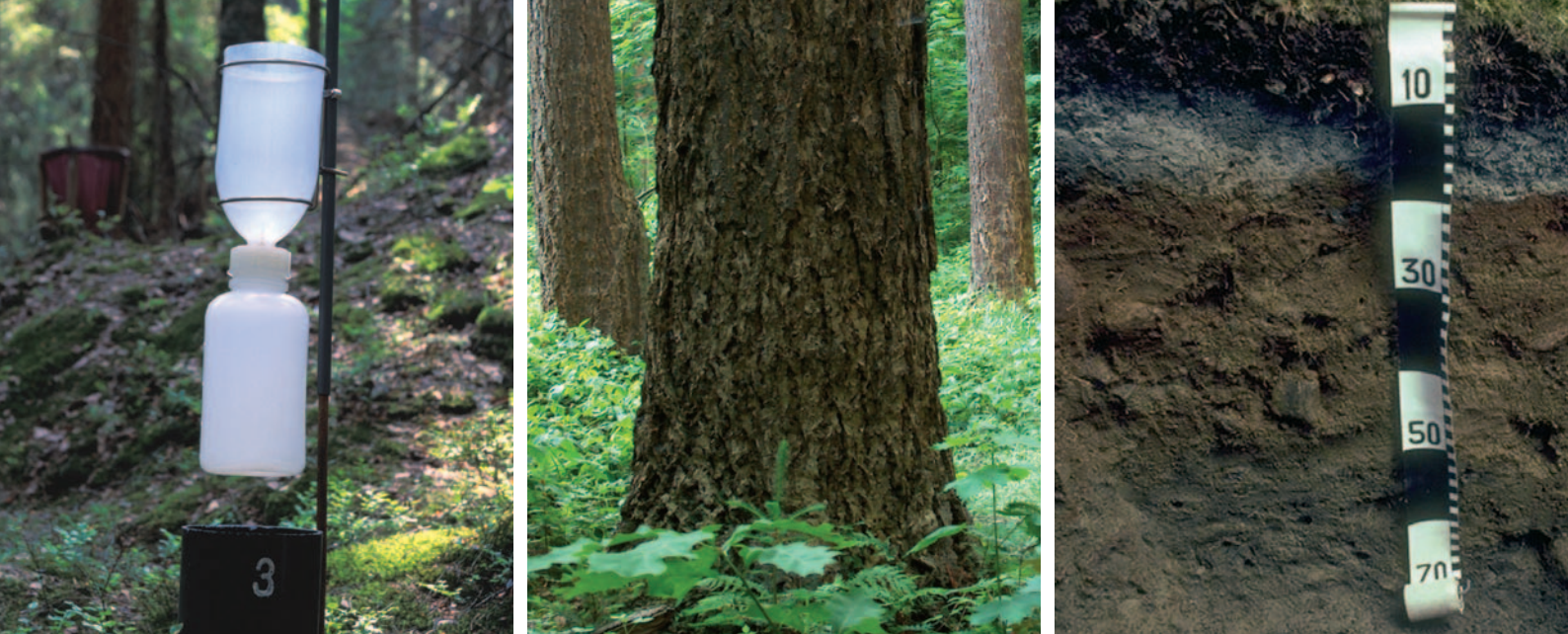
Deposition measurement equipment (left), tree stems (middle), and soil profile (right). Key processes included in dynamic soil chemistry are element fluxes in deposition, nutrient uptake by trees, and nutrient cycling in the soil.
